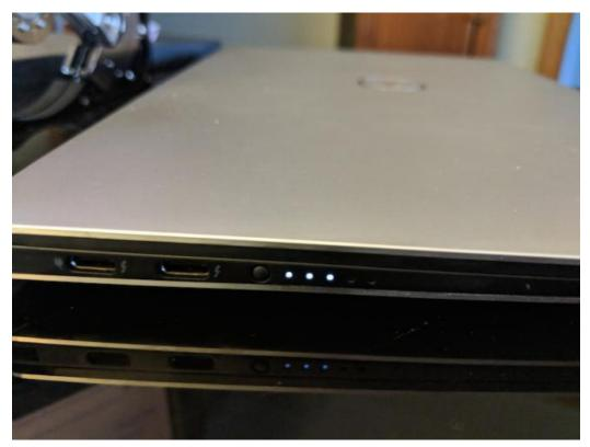
Figure 3. The Visual Battery Indicator
