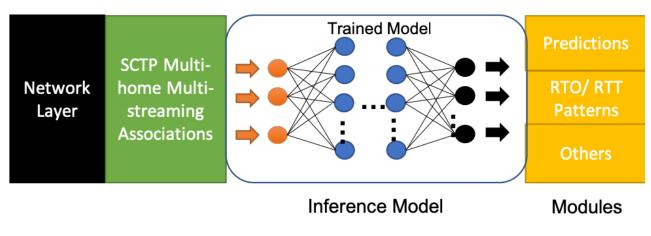
Figure 2. Inference model implementation: RTT/RTO values from SCTP are fed to an inference model to produce smarter congestion handling.
