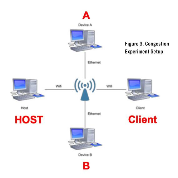
network to evoke congestion. Figure 3 shows the system designations, where A/B systems provided cross traffic and are connected via wired Ethernet, and Host/ Client systems provided test data and are connected via wireless. In this scenario, 5,000 15-second samples were collected from the Client node as it sent SCTP-Test packets to the Host node, while A-to-B traffic consisted of 1MB, 512KB, 256KB, 128KB and 1KB chunk size FTP traffic.
