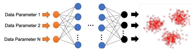
Figure 1. Deep learning neural network: orange nodes are the input layer, blue nodes are hidden layers, and black nodes are the output layer. The red circles on the far right are outputs that have been "clustered" by the network.
