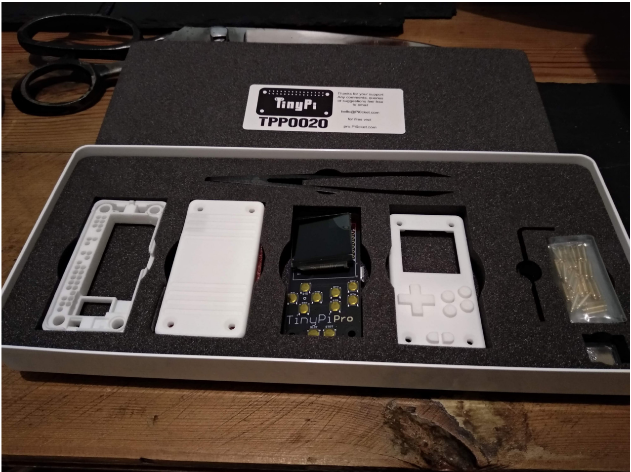
Figure 3. The parts of the TinyPi—the Smallest Handheld Game Console I Can Possibly Imagine
