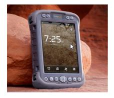
The new RAMPAGE 6 rugged notepad with Android is the result of a collaboration between Juniper Systems and SDG Systems. The RAMPAGE 6 is a unique iteration of Juniper Systems' Mesa Rugged Notepad, which features a 5.7-inch viewing display, IP67 ingress protection rating for water and dust, integrated 2–5 meter GPS receiver, optional integration of a 1D/2D barcode scanner, and optional Class I, Division 2 certification for use in hazardous
