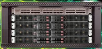
Microway MD SimCluster with 8 Tesla M2090 GPUs 8 Intel Xeon E5 CPUs and InfiniBand 2X Improvement over Xeon 5600 Series
