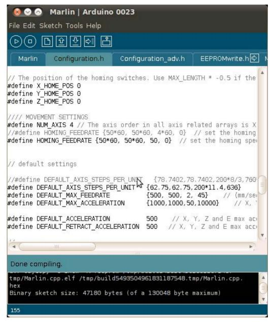
Figure 1. Marlin Configuration with Arduino Software
