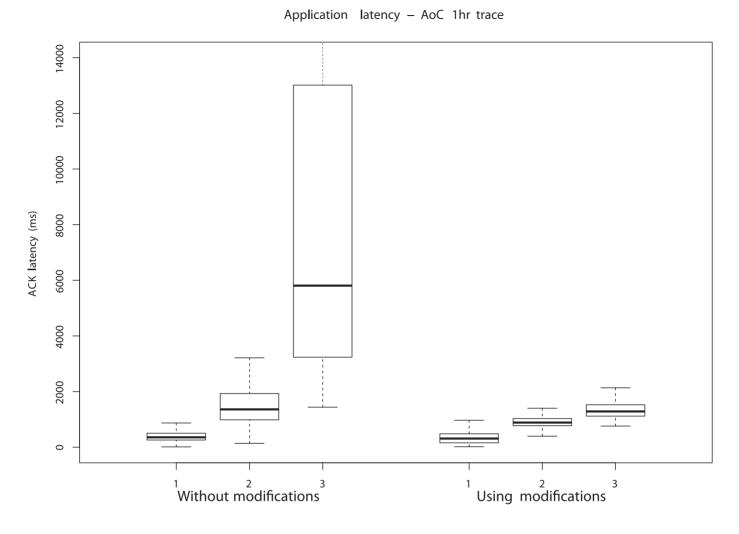
Figure 4. Modified vs. Traditional TCP in *Age of Conan*. The box shows the upper and lower quartiles and the average values. Maximum and minimum values (excluding outliers) are shown by the drawn line. The plot shows statistics for the first, second and third retransmissions.
