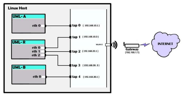
Figure 2. The Three UML Machines Once Booted Up
