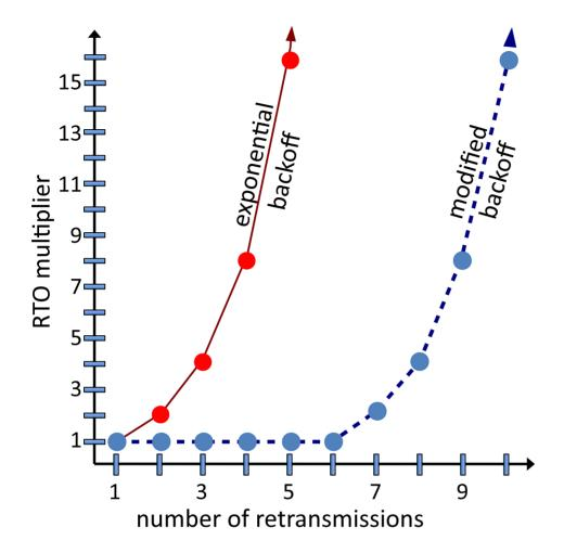
Figure 3. Modified and Standard Exponential Backoff
