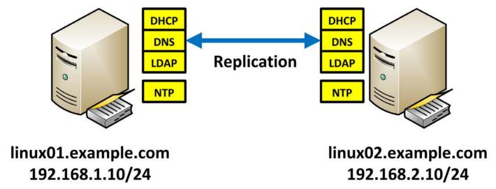
Figure 1. Example redundant server pair—in Part I of the series, NTP, DNS and DHCP were configured.
