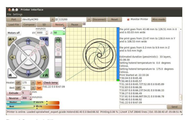
Figure 3. Pronterface's GUI
