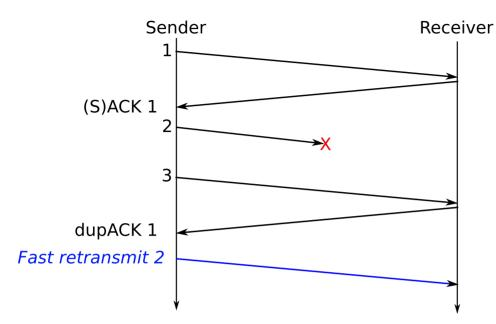
Figure 2. Thin Fast Retransmit
