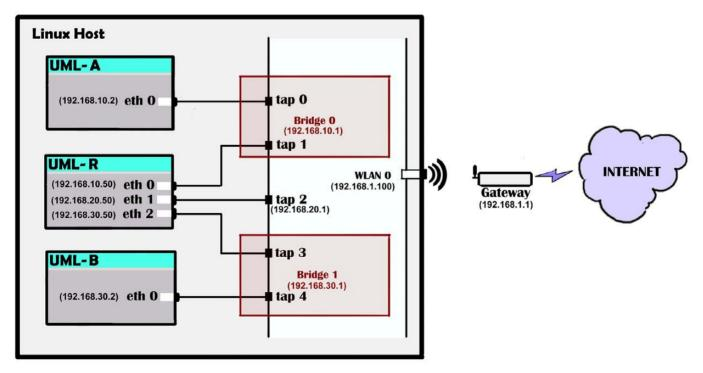
Figure 4. UML Machines, after Executing the setup\_network\_connections.sh Script
