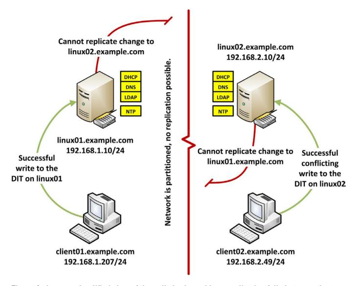
Figure 2. An over-simplified view of the split-brain problem: replication fails between the two servers despite the local network still being available.
