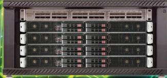
Microway MD SimCluster with 8 Tesla M2090 GPUs 8 Intel Xeon E5 CPUs and InfiniBand
