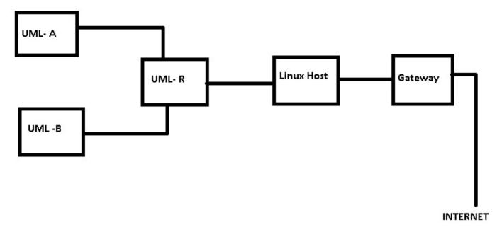
Figure 1. High-Level Block Diagram of the Example UML Setup
