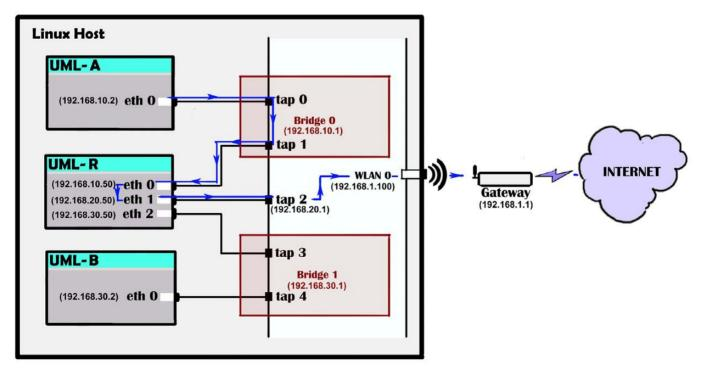
Figure 5. Packet Flow in the UML Network
