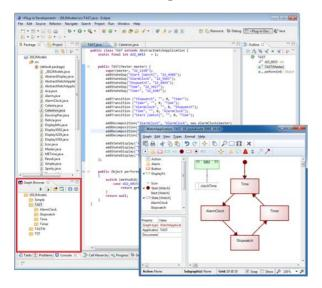
Eclipse, and it automatically imports source code generated from the MetaEdit+ models into Eclipse and builds and runs it there. Traditionally, development teams have found it difficult to combine the use of models and code due to the modeling languages used and the programming environments. Now, with the plugin, however, the domain-specific models—expressed as diagrams, matrices or tables in MetaEdit+—can be browsed and used directly from Eclipse. http://www.metacase.com
