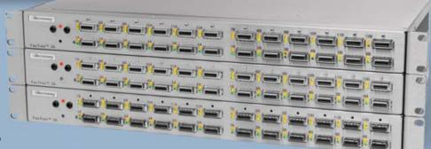
24 instead of 12, improving nearest neighbor latency in fine grain problems and doubling the size of the largest three hop fat tree that can be built, from 288 to 576 ports. Larger fabrics can be created linking 576 port domains together.
